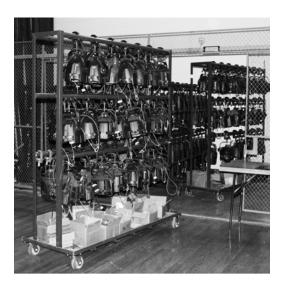
THIS PARTICULAR RACK HAS THREE HANGING PIPES BECAUSE SOURCE FOUR PARS ARE SMALLER THAN MOST OTHER TYPES OF LIGHTS It is a good idea to provide a plywood bottom to the rack for gel frames and barn doors and the like. You may wish to use two swivel and two rigid casters if the racks must travel long distances with one person pushing them. If they must be maneuvered through tight spaces, four swivel casters will probably work better.
